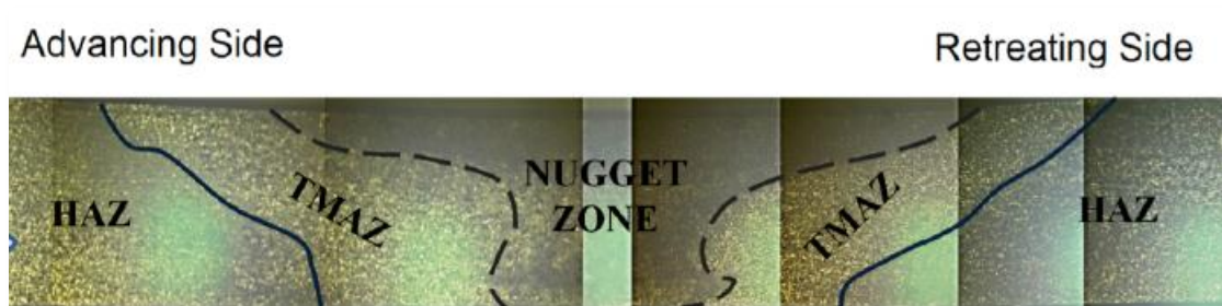
Fig.(5) Schematic of FSW & FSP primary zones
