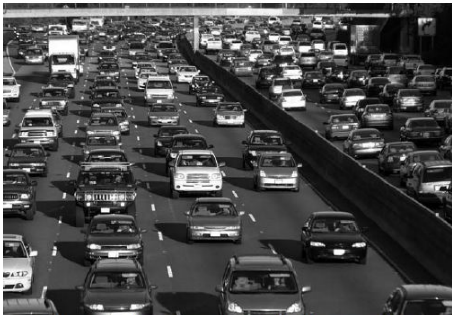
(b) In this case, vehicles shy away from the roadside barrier. This causes the placement of vehicles in each lane to be skewed toward the median. This is also an indication that the median barrier illustrated here does not present an obstruction to drivers.
