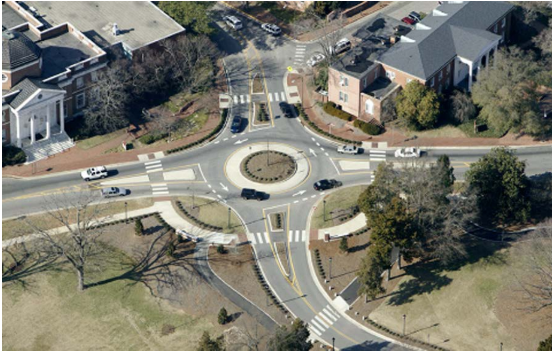
Figure: Yield-controlled intersection (modern roundabout).
