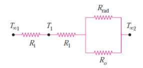
The thermal resistance network for this problem is given in figure 2–15. Noting that the inner diameter of the tank is D1 = 3 m and the outer diameter is D2 = 3.04 m, the inner and the outer surface areas of the tank are
