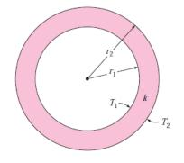
Figure 2-12 A long cylindrical pipe (or spherical shell) with specified inner and outer surface temperatures *T*1 and *T*2.
