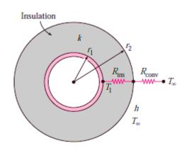
Figure 2-16 An insulated cylindrical pipe exposed to convection from the outer surface and the thermal resistance network associated with it.
