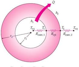
$R_{\text{total}} = R_{\text{conv},1} + R_{\text{cyl}} + R_{\text{conv},2}$
