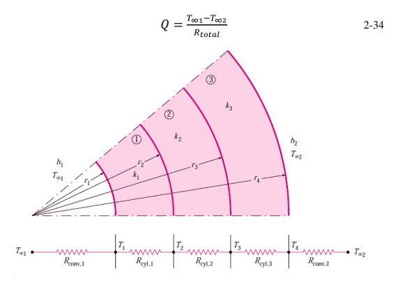
Figure 2-14 The thermal resistance network for heat transfer through a three-layered composite cylinder subjected to convection on both sides
