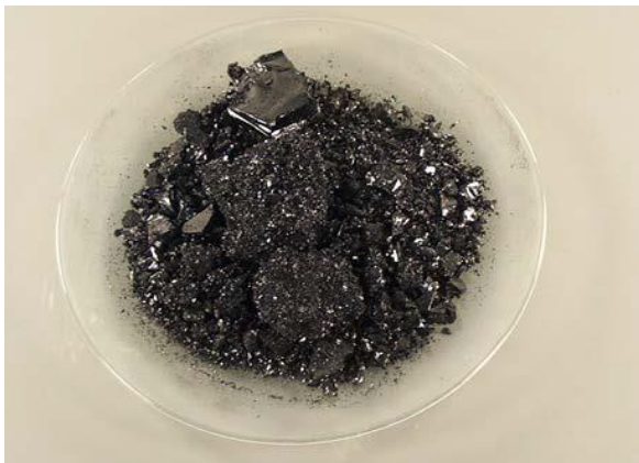
Hard (Low penetration)
