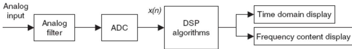
FIGURE 1.4 Signal spectral analysis.
