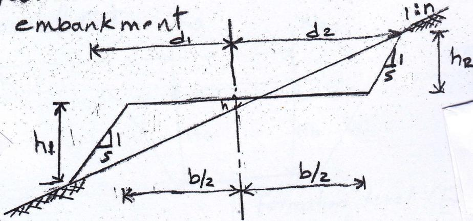
(B) When the center line of the formation is in excavation
