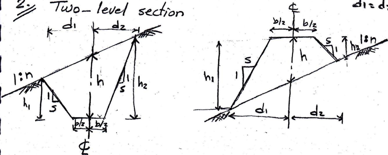
(n) is the lateral slope of the original ground surface
