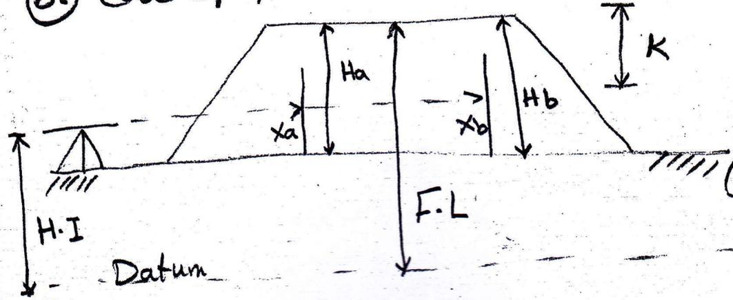
$$\begin{aligned} F.L - H.I &= K \\ H_a &= K + x_a \\ H_b &= K + x_b \end{aligned}$$
