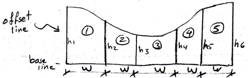
$$\text{Area of } \textcircled{1} = \frac{h_1+h_2}{2} \times W, \text{ Area of } \textcircled{2} = \frac{h_2+h_3}{2} \times W, \dots$$
