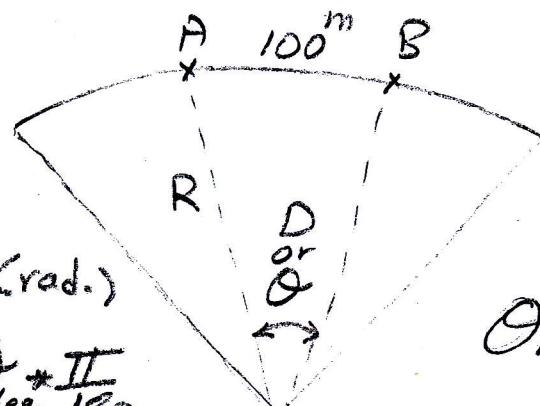
2. Chord definition ( $\theta_c$  or D) : is an angle subtended at the center of the curve by chord having a length of 100 m.
