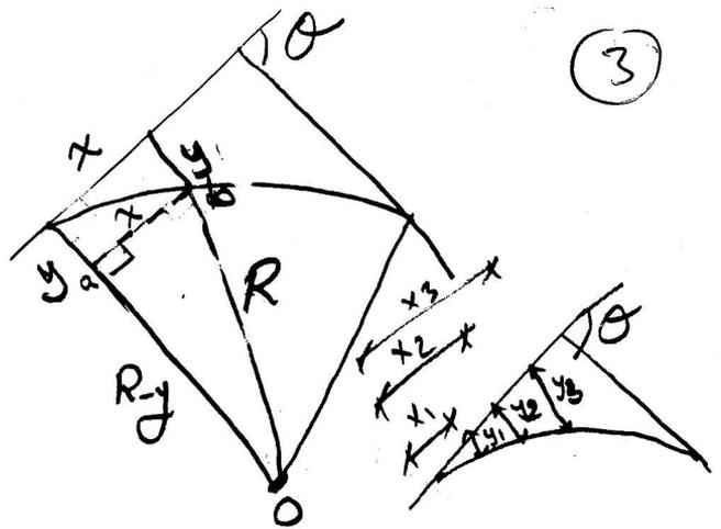
The curve is set out in two parts, starting from each tangent.
