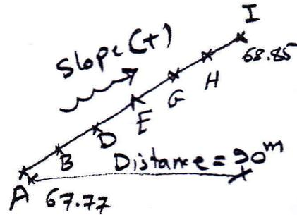
$$\text{slope)}_{A \rightarrow I} = \frac{\text{grade)}_I - \text{grade)}_A}{\text{Distance}} = \frac{68.85 - 67.77}{90} = +0.012$$
