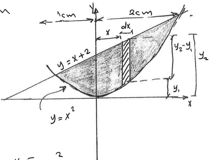
The mom. of the element with respect to y-axis
