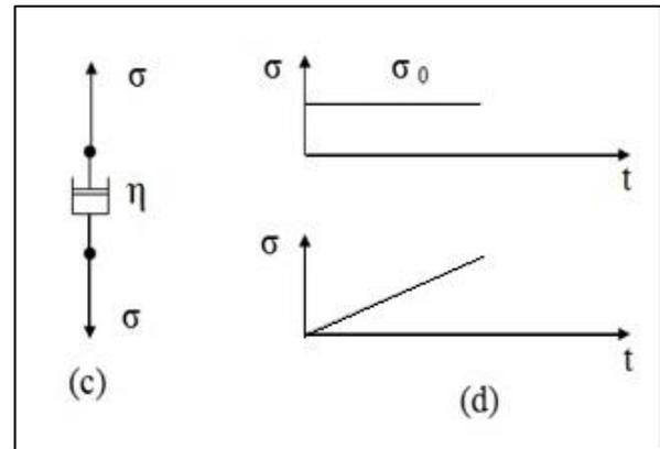
Figure Behavior of linear dashpot
