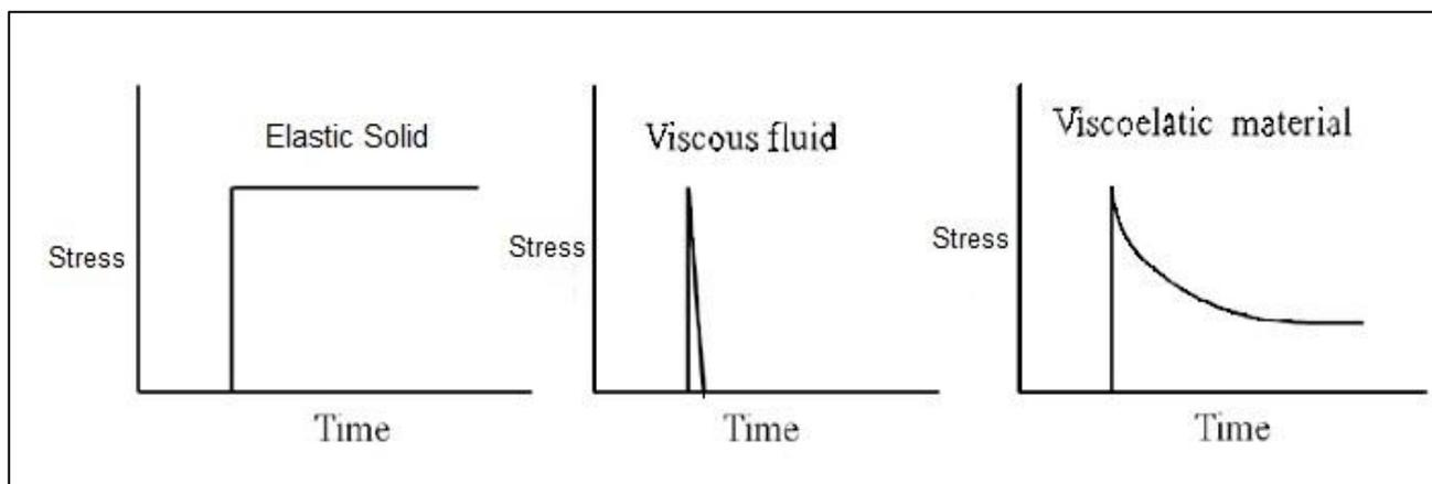
Figure ,Stress relaxation behavior of three different types of materials subjected to same amount of strain.
