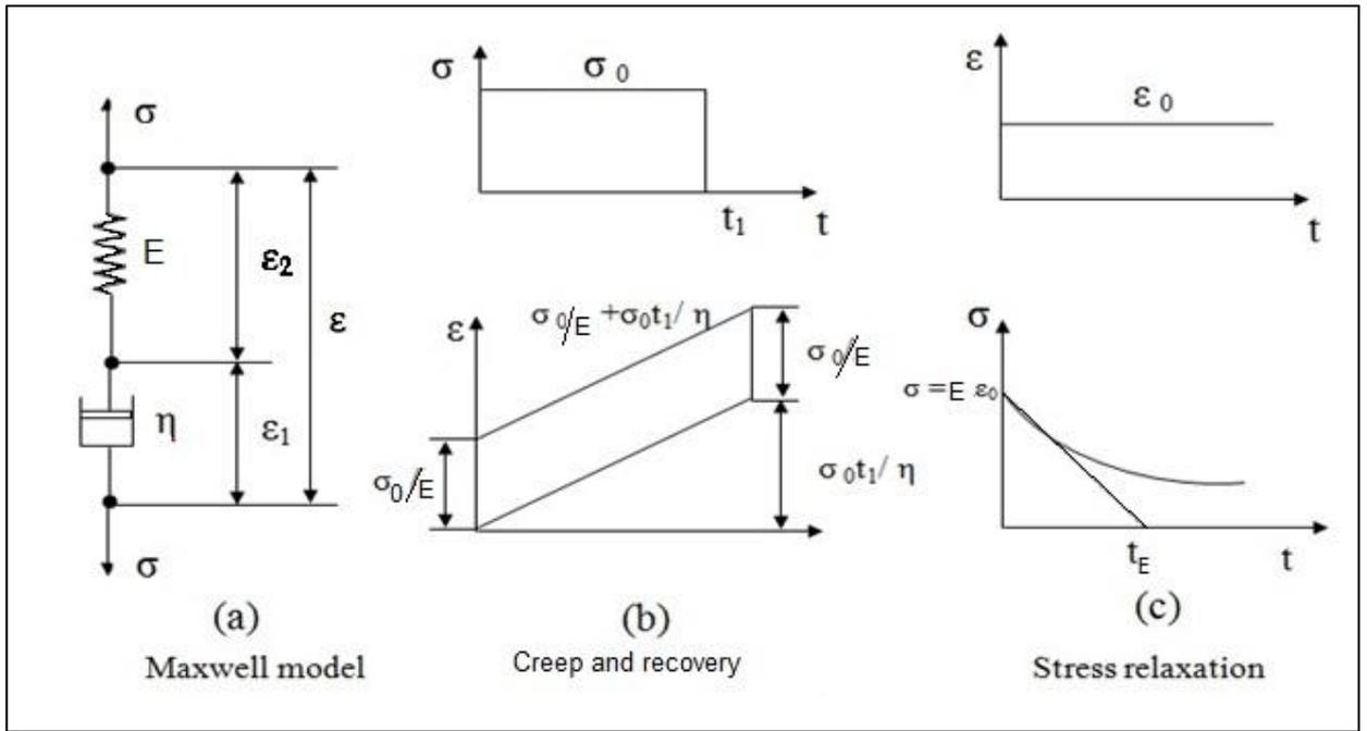
Figure Behavior of Maxwell model
