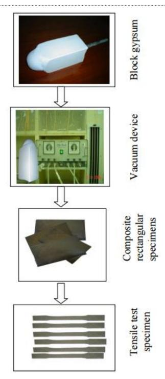
The method of preparation of composite specimen is called vacuum method to prevent defects and cavities which follow by:
