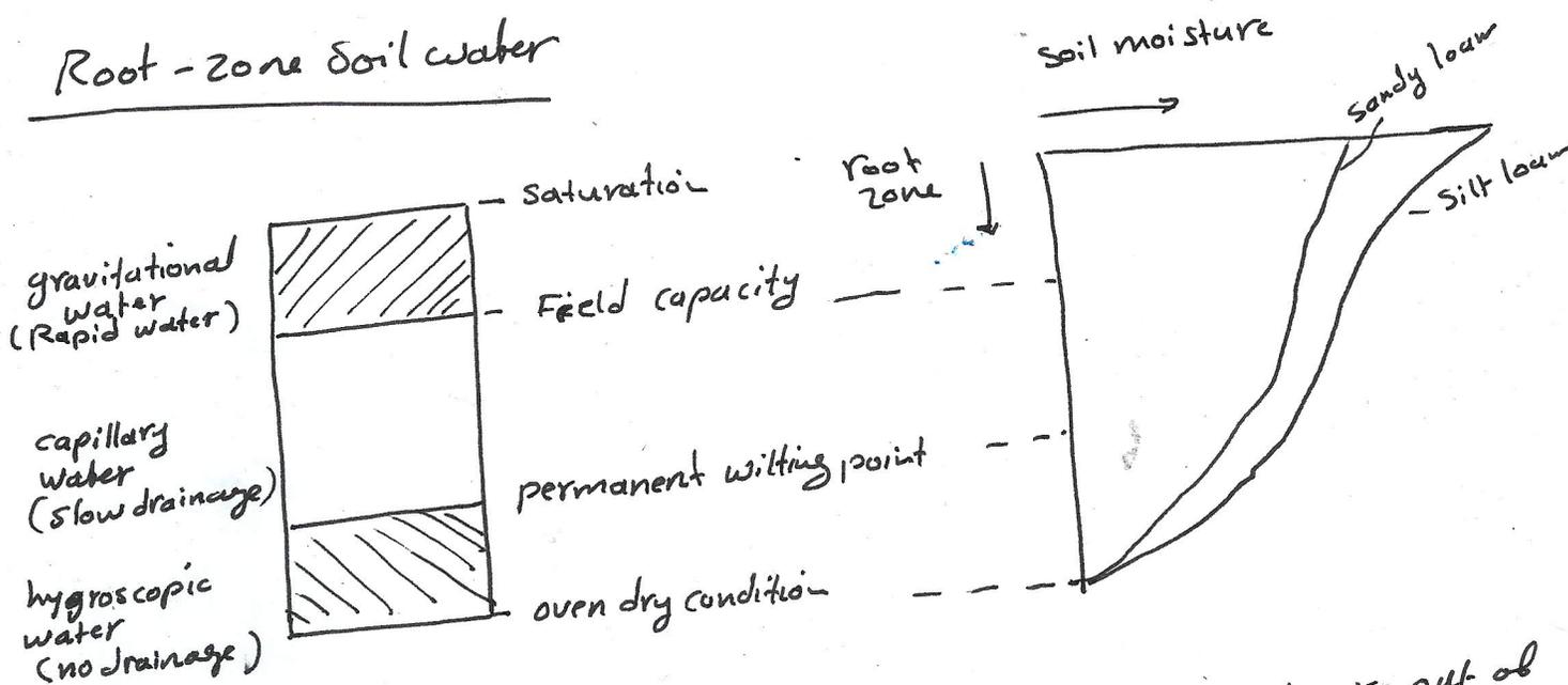
Gravitational water: the water that moves into, through or out of the soil by gravity
