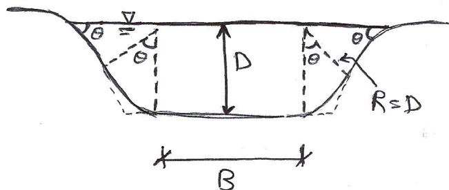
Ex. Design a lined canal of discharge  $120 \text{ m}^3/\text{s}$ . The permissible velocity of flow is taken as  $2 \text{ m/s}$ . Assume side slope  $1:1$  and  $n = 0.018$  whereas the slope of the canal is  $1/3000$ .
