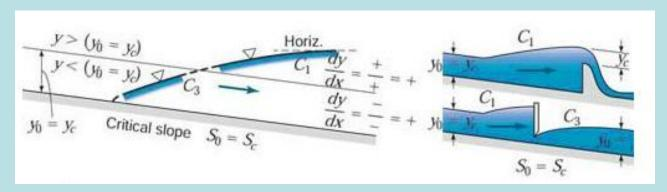
$$\frac{dh}{dx} = S_f \frac{1 - \left(\frac{q^2}{h^3 C^2 S_f}\right)}{1 - \frac{q^2}{gh^3}} = S_f \frac{1 - \left(\frac{h_n}{h}\right)^{10/3}}{1 - \left(\frac{h_c}{h}\right)^3}$$
