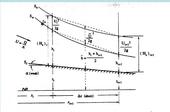
Fig. 4.3 Scheme of a non-uniform flow between two cross sections.
