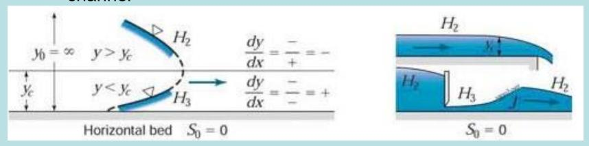
$$\frac{dh}{dx} = S_f \frac{1 - \left(\frac{q^2}{h^3 C^2 S_f}\right)}{1 - \frac{q^2}{gh^3}} = S_f \frac{1 - \left(\frac{h_n}{h}\right)^{10/3}}{1 - \left(\frac{h_c}{h}\right)^3}$$
