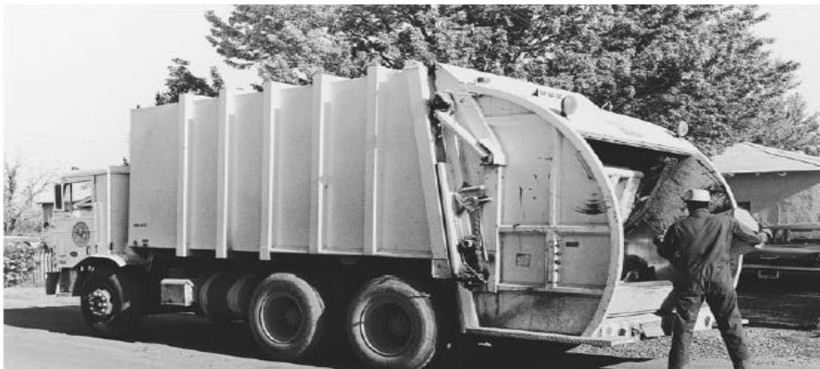
Fig.1. Collection of wastes from containers placed at curb by homeowner (a) with a side-loading vehicle equipped with a right-hand drive mechanism, and (b) with rear-loading collection vehicle. The rear-loaded type of collection vehicle is commonly used with two- and three- person crews for the collection residential wastes in many parts of the United States.
