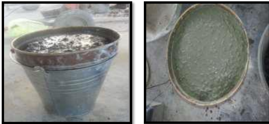
Fig (9): Sieve segregation resistance test using standard sieve (diameter of square hole: 5mm, diameter of the sieve: 350mm)
