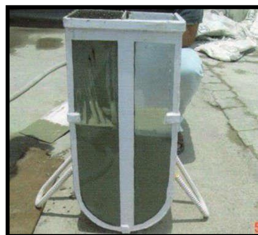
Fig. (8): U-Box test instrument and procedure.
