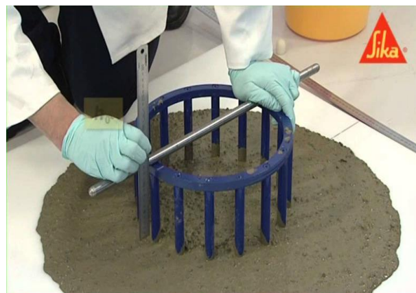
Fig. (5): J-Ring test instruments and procedure.
