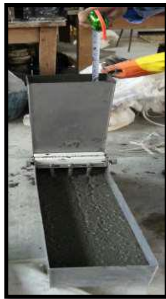
Fig. (6): L-Box test instrument and test procedure
