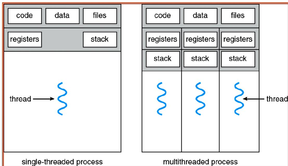
Figure 6.1 Single-threaded and multithreaded processes.
