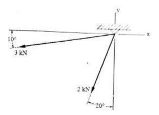
2- Determine the magnitude and direction of the resultant of the forces shown in the figure below.
