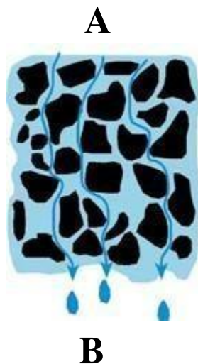
Fig.(1): Water Path Through Soil Voids
