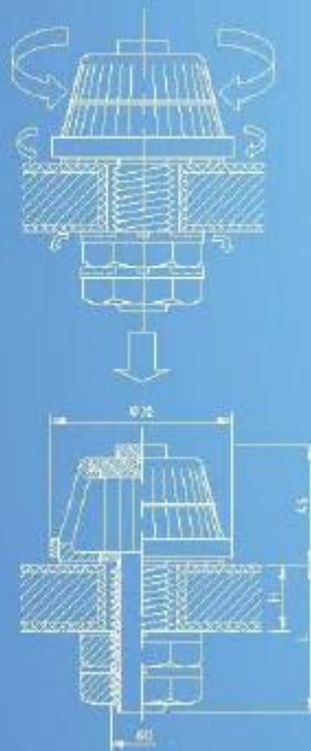
Figure (7.10): Rapid sand filter perforated slab and nozzle under-drain
