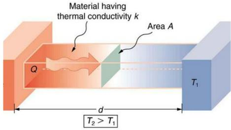
The amount of heat transferred through unit area of specimen with unit thickness in unit time is termed as thermal conductivity. It is measured in kelvins. It depends on material structure, porosity, density and moisture content. High porous materials, moist materials have more thermal conductivity
