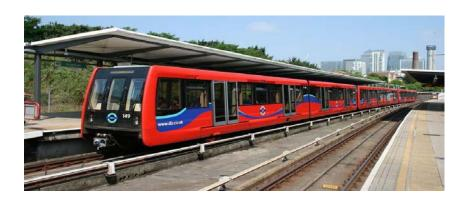
• Rubber-tired rapid transit consisting of moderately large vehicles, supported or guided by rubber tires running on wooden, steel, or concrete surface.
