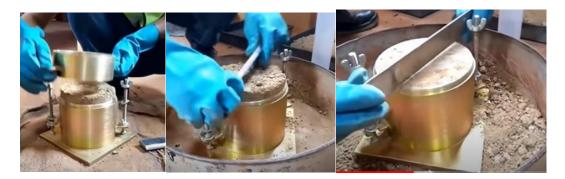
12. Weigh and record the (weight of mold +wet soil )
