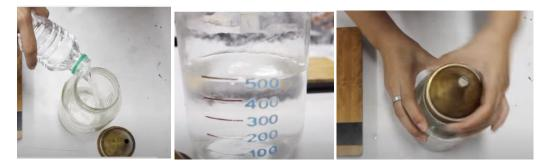
4. Record the weight of pycnometer +water (Wa)
