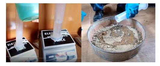
6. Mix the soil thoroughly. Divide the processed soil into parts.
