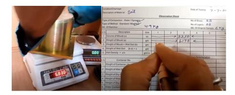
13. Weigh the empty container and record the weight in the lab sheet
