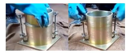
8. Take an amount of the processed soil, and hence place it in the mold in 3 or 5 equal layers (based on the selected method). Take the first portion and compact it by giving 25 or 56 blows of the rammer (based on the selected method). The blows should be uniformly distributed over the surface of each layer.
