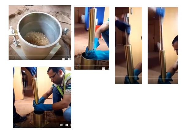
9. The second layer should also be compacted by the same number of blows of rammer. Likewise, place the remaining layers and compact them.
