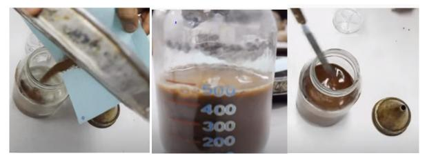
7. Weigh the water + soil + pycnometer (Wb)
