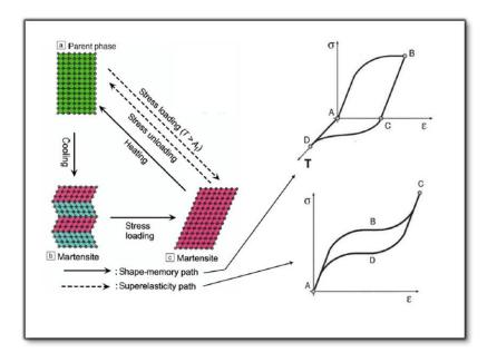
Shape memory alloys have two phases namely austenite and martensite; Austenite is the high temperature or "parent" phase .
