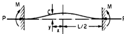
Figure 8.4: - Strut with fixed ends.
