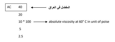
Thus, AC-5 (viscosity is 500  $\pm$  100 poise at 60° C (140° F)) is less viscous than AC-40 (viscosity is 4000  $\pm$  800 poise at 60° C (140° F)).
