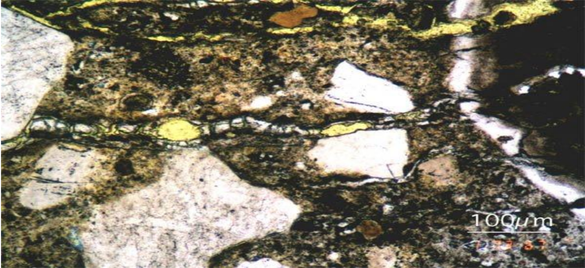
Figure 2 Concrete thin-section, viewed with a petrographic microscope, showing a chert aggregate particle (at the right of the image) from which alkali-silica gel has extruded into adjacent cracks.
