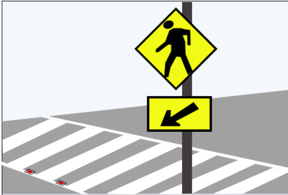
Figure 16: In-Pavement Raised Markers with Amber LED Strobe Lighting and LED Signs.
