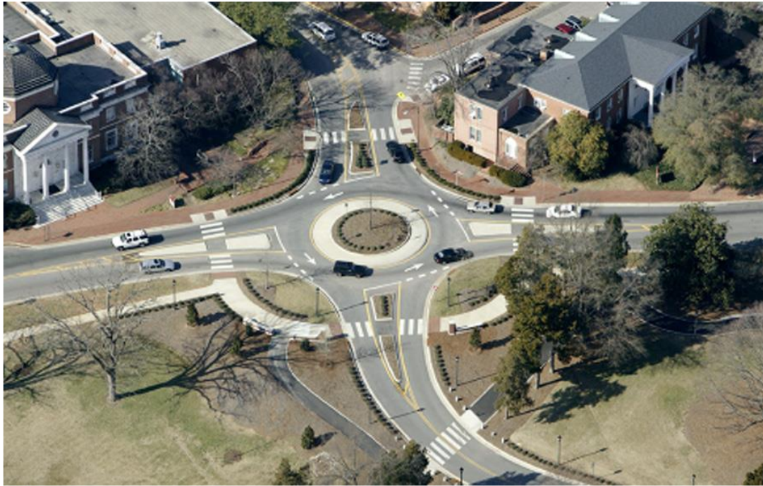
Figure: Yield-controlled intersection (modern roundabout).
