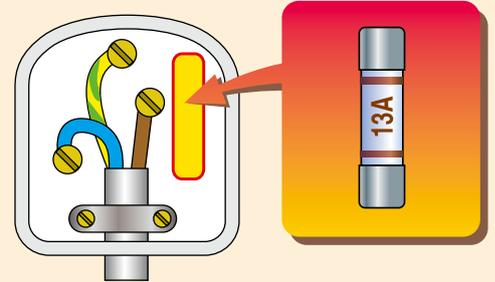
**A fuse must be installed on “live” wires.** When replacing a fuse, the new fuse must be same current fusion value as the old one.
