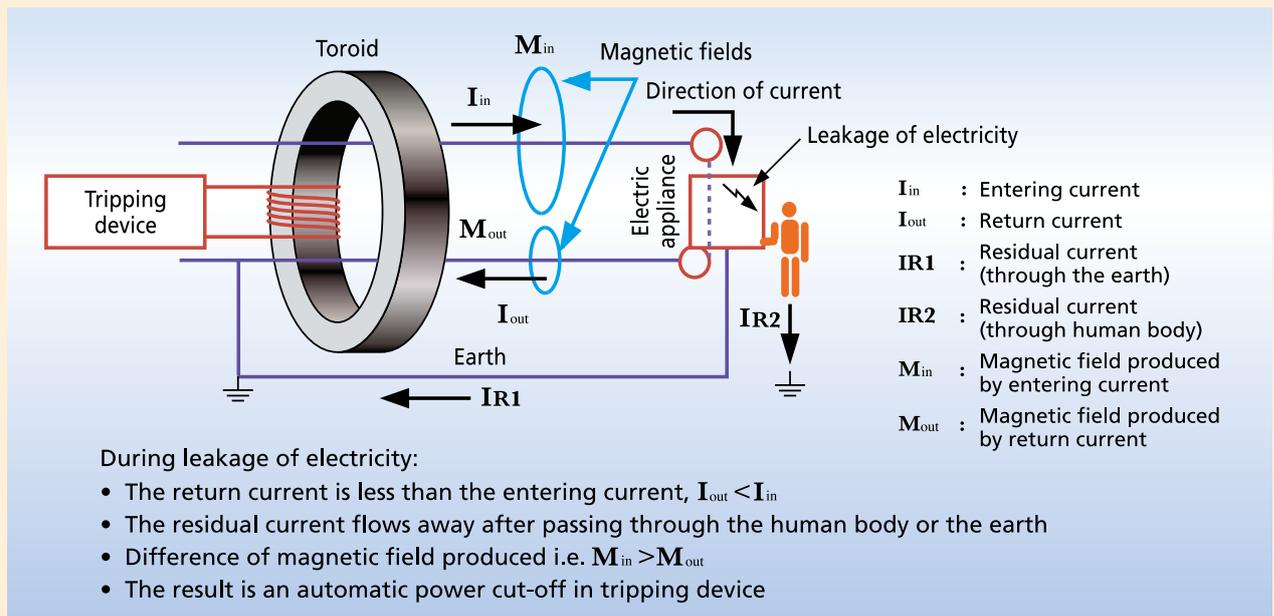
If ELCB is not fixed in main circuit box or the worker works in high risk environment (E.g. humid condition), portable RCD(Residual Current Devices) should be installed to reduce the chance of getting an electric shock.
