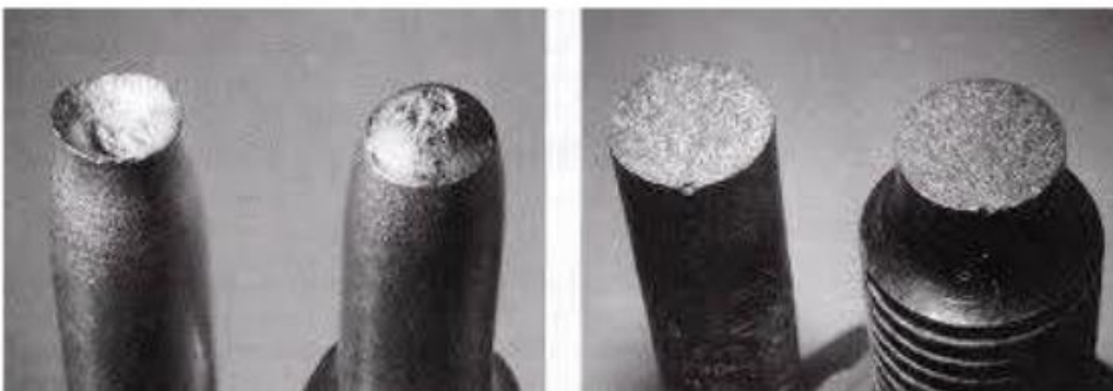
(a). Cup & Cone Ductile Fracture;
