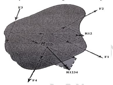
The resultant is a couple when the resultant of all but one of the forces of the system and the remaining force form a couple.
