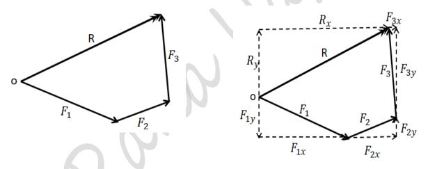
We will find out the resultant force for many forces acting on a rigid body by using the following equations:-
