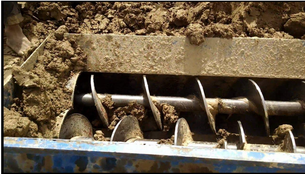
Fig. 4: Clay mixing with water
