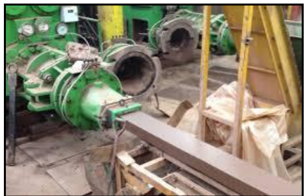
Fig. 3: Molding of clay bricks
