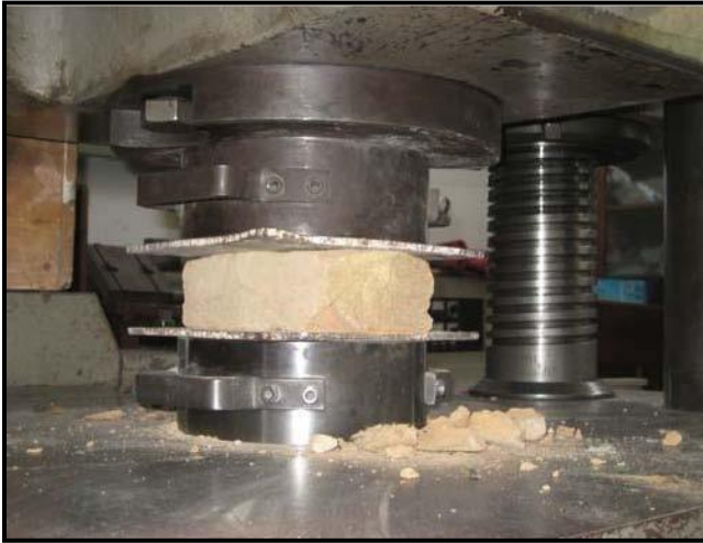
Fig. 6: Compressive strength machine.
