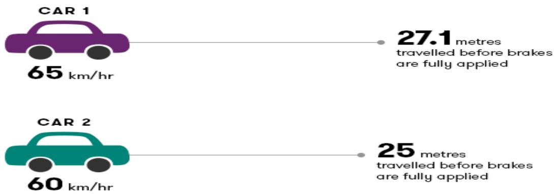
**reaction distance:** Due to the delay in human reaction, however, there is always a time *lag* between seeing a hazard and braking the car. This time interval is known as ***reaction time***, which is vary widely for different persons. During the reaction time the car travels a distance known as ***reaction distance***.
