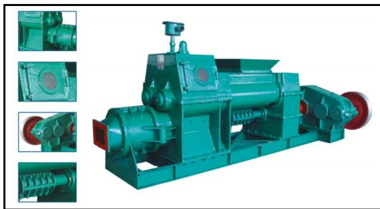
Fig. 5: Clay brick extrusion machine (CBM 26/08)
