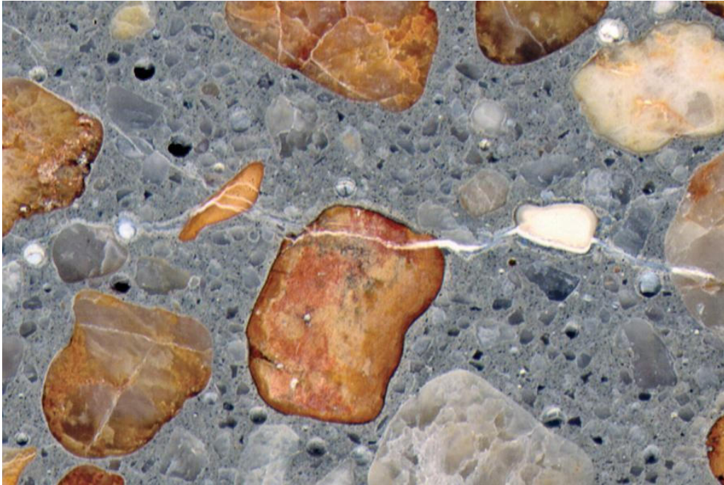
Figure 2 Concrete thin-section, viewed with a petrographic microscope, showing a chert aggregate particle (at the right of the image) from which alkali-silica gel has extruded into adjacent cracks.
