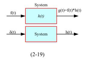
where h(t) is called the impulse response of the system, h(t) is found by applying  $\delta(t)$  at the system input, where the output would be h(t),
