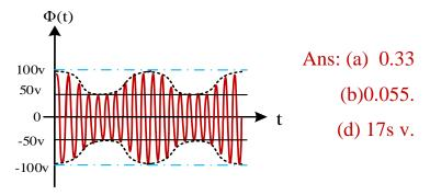
**Q2:** A given AM (DSB – LC) transmitter develops an unmodulated power output of 1 kW. Across  $50\Omega$  resistive load. When a sinusoidal test tone with a peak amplitude of 5v is applied to the input of the modulator, it is found that the spectral line for each sideband in the magnitude spectrum for the output is 40% of the carrier line. Determine the following quantities in the output signal:
