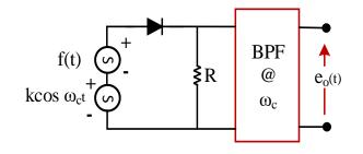
In this case the nonlinearities in the diode characteristics may be approximated with the power series of the form:
