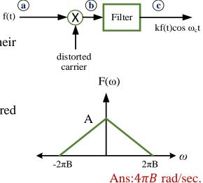
**Q22:** Show that the scheme shown in fig. Below can be used to generate DSB-SC signal. Assuming that f(t) is a signal bandlimited to B Hz, find the signals and sketch their spectra at points a, b, c and d. Explain the nature of filter in this figure.
