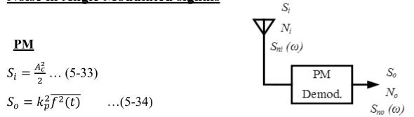
If the channel noise is white and double-sided PSD is  $\eta/2$  watt/Hz. Then PSD at the demodulator output is:
