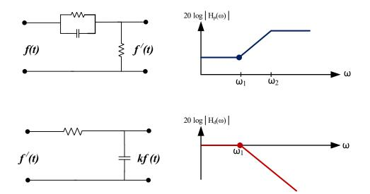
The frequency  $f_1$  is 2.1 kHz and  $f_2$  is typically 30 kHz or more, the preemphasis transfer function is:
