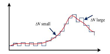
If the step size adaptation is made in continuous form with slope of the input, then the name CVSDM (continues variable slope DM) is used, or it is made in discrete form with finite number of step size to form discrete variable slope DM. In the CVSDM, peak detector circuit are used to control  $\Delta V$ , while in discrete VSDM logic circuit are used to control  $\Delta V$ .
