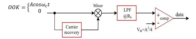
Here, a carrier recovery circuit is required to generate the carrier signal cos  $\omega_c t$  then, the LPF will cutoff of  $\mathbf{R}_b$  is used to give the high and low states of the data.
