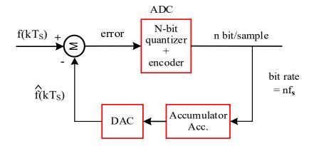
At the Rx, the accumulator (Acc.) will integrate DPCM signal to produce  $\hat{f}(kT_s)$  to DAC output then smoothed using LPF.
