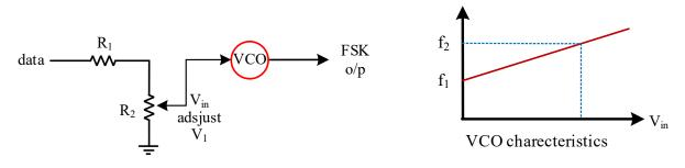
A voltage-controlled oscillator is usually used for FSK modulation. A VCO is an oscillator with an internal tuning capacitor, which controlled by an external voltage  $V_{in}$ . This capacitor is called varicap (\_\_\_\_\_\_).
