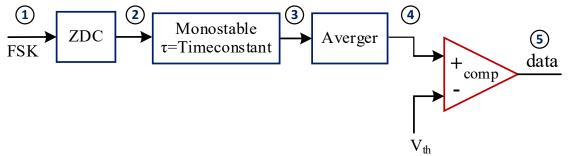
$V_{th}$  The zero crossing detector (ZDC) changes sinewave into rectangular waves with frequencies  $f_1$  and  $f_2$ .
