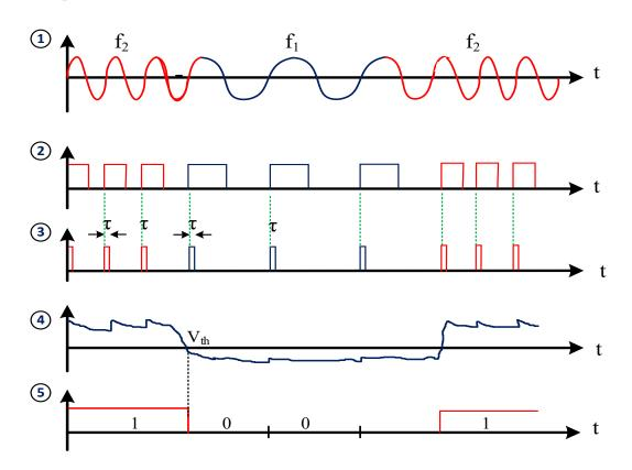
The positive going edge monostable gives fixed time constant  $\tau$  chosen such that  $\tau \leq (\frac{1}{f_2})$ . The average value of the monostable output is high level for frequency  $f_2$  and is low level for frequency  $f_1$ . A threshold comparator with a threshold V<sub>th</sub> chosen midway between the high & low value will give data output.
