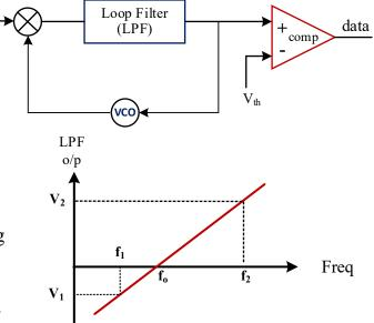
$$V_{th} = \frac{V_1 + V_2}{2} \qquad \dots (6-27)$$
