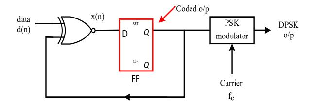
The coded output x(n) is obtained from transmitted data using:
