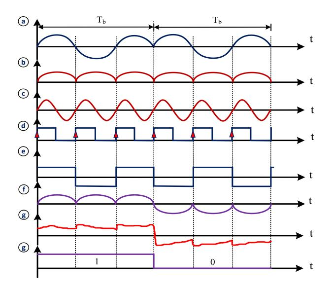
The  $\pm A \cos \omega_c t$  PSK modulation is first canceled using squarer to give  $\frac{A^2}{2}(1 + \cos \omega_c t)$ , the double carrier frequency is filtered using BPF tuned at  $2\omega_c$ , then T-FF is used to generate carrier at  $\omega_c$  with correct phase.
