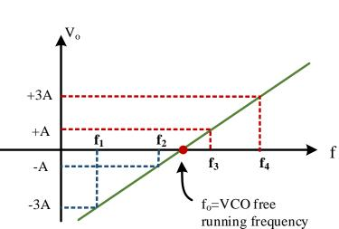
(M-1) threshold comparators (3 comparator here) will give  $C_1$ ,  $C_2$  &  $C_3$  output and in a similar schematic as in MASK these outputs will be decoded into the received data (V<sub>th</sub> are -2A, 0, +2A).
