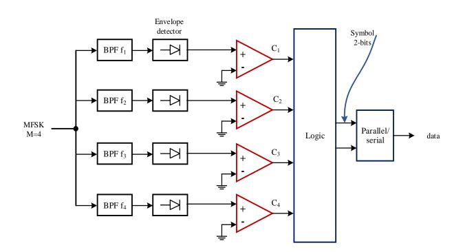
Note that only once of the envelope detectors is high during  $T_s$  time, corresponding to one of the received frequencies  $f_1$ ,  $f_2$ ,  $f_3 \& f_4$ .
