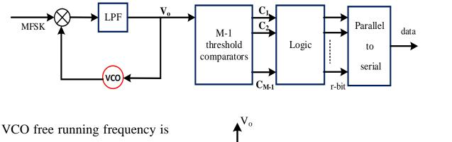
chosen midway between  $f_2$ &  $f_3$ (center of the band). Suppose that the liner region of PLL gives  $V_0$ = -3A, -A, +A & +3A, corresponding to  $f_1$ ,  $f_2$ ,  $f_3$ &  $f_4$ respectively.
