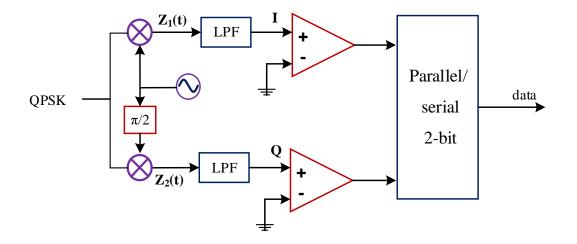
$$Z_{1}(t) = \pm A\cos^{2}\omega_{c}t \pm A\sin\omega_{c}t \cos\omega_{c}t \implies I = \pm A$$
