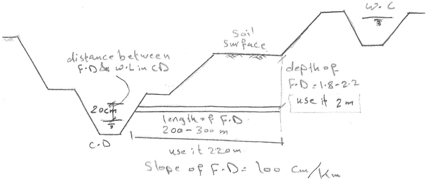
$$W.L_{CD} = G.L - \text{depth of field drain below G.L} - S_{FD} \times L_{FD} - \frac{S_{CD} \times L_{CD}}{\text{distance from F.D to w.l.in C.D}}$$
