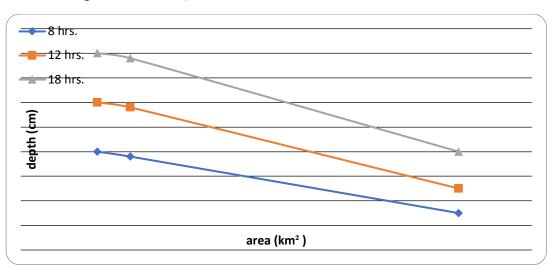
The depth of rainfall in the center of the catchment is the maximum rate and it decreases with the area, increasing (at area =0, P = maximum)
