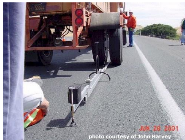
Figure 19. Benkelman beam in use
