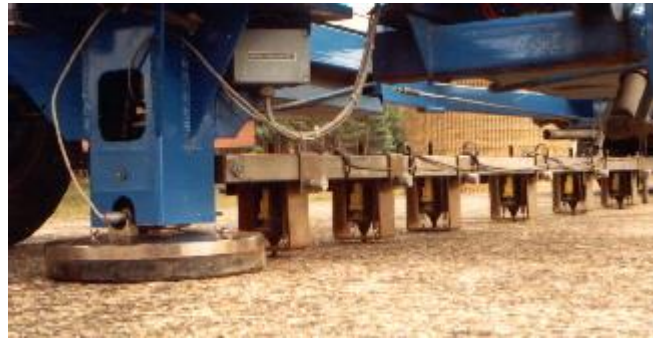
Figure 24. FWD impulse loading mechanism (foreground) and sensors (background).
