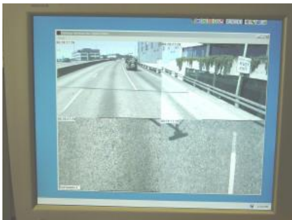
Figure 11. Pavement condition rating video images.
