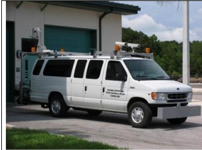
Figure 7. South Dakota Road Profiler (van-mounted)
