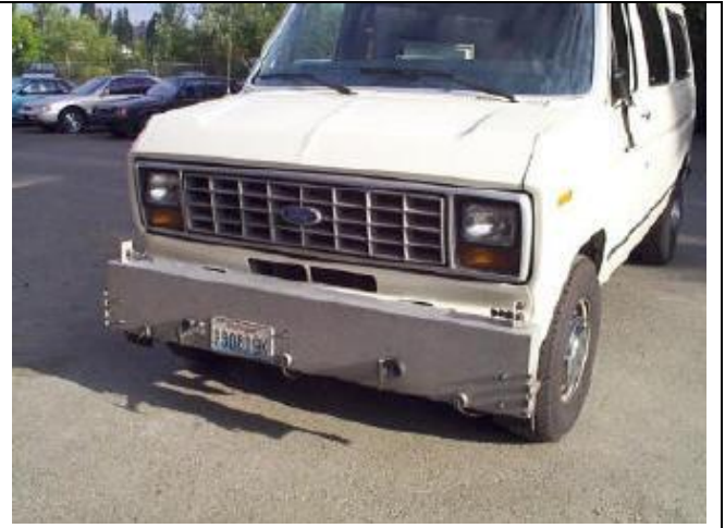
Figure 8. Imaging survey van used by the state materials office of the Florida DOT. The profiler is the grey/silver box attached on the front bumper
