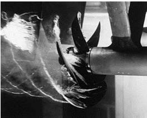
Cavitating propeller model in a water tunnel experiment.
