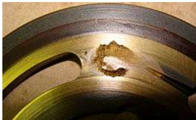
Cavitation damage on a valve plate for an axial piston hydraulic pump.
